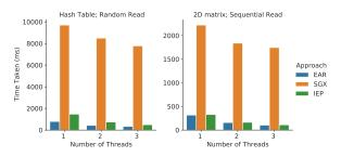
Figure 2: Time to complete a summation for values in a hash table and 2D matrix vs. number of threads for a data set that occupies 512MB (~5x EPC size). SGX's paging performance does not scale in thread count for large data sets as page fault synchronization serializes threads.
