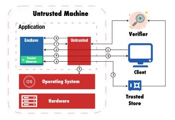
Figure 1: A high-level view of EAR's architecture. Solid arrows denote authenticated, integrity-protected communication; dashed arrows are procedure invocations.
